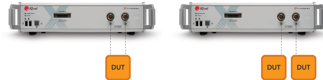
Figure 4a: IQxel-160 testing an 80 MHz, 802.11ac, 2x2 MIMO device using True-MIMO method
