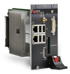
Trigger: bi-directional external trigger port (SMB) Dual GbE ports Four USB 2.0 ports DVI display connector ExpressCard/34 expansion slot Micro-D GPIB connector
