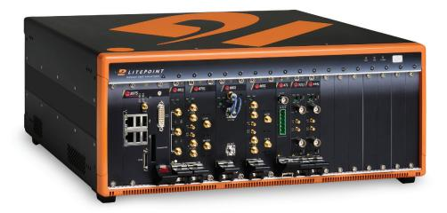
The LitePoint zSeries 18-slot chassis is an 18-slot PXI Express chassis, compliant with PXI Express and cPCI Express specifications and offering one system slot, one system timing slot, ten hybrid peripheral slots, and six PXI Express peripheral slots for a wide variety of testing and measurement applications requiring enhanced bandwidth.
