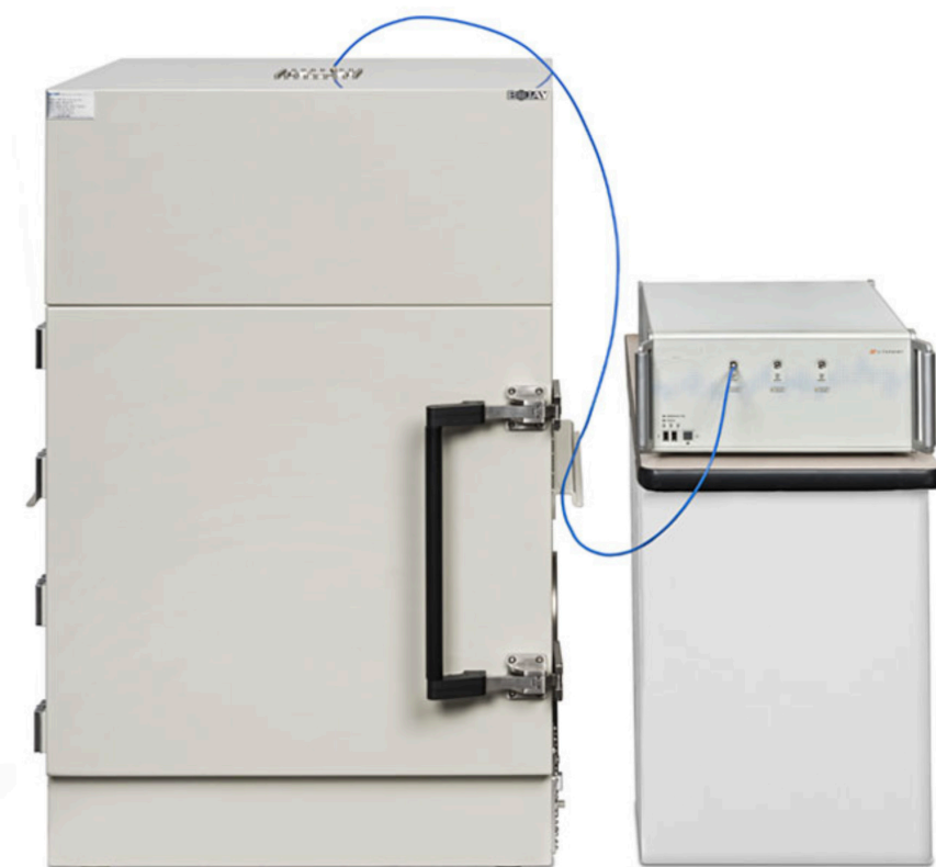
Figure 3. A 60-cm DFF OTA chamber is shown with LitePoint's IQgig-5G mmWave tester.
