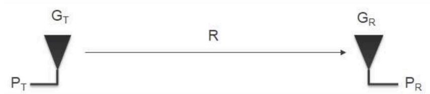
Figure 4. Setup variables required to calculate the OTA link budget using Friis equation.
