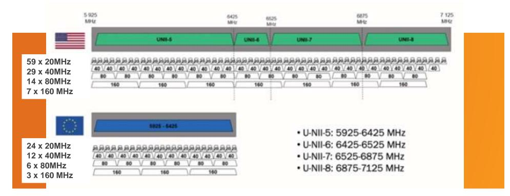
Some frequency bands may require reduced power for incumbent protection Some bands may required AFC (Automated Frequency Coordination) for incumbent protection
