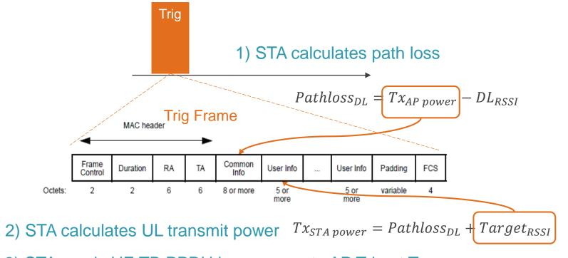
3) STA sends HE TB PPDU in response to AP Trig at Tx STA power
