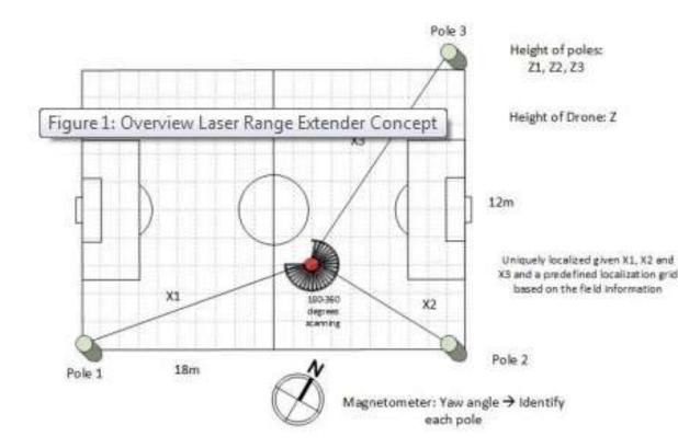
In a **2-dimensional world**, with 3 distance measurements you can accurately determine location.
