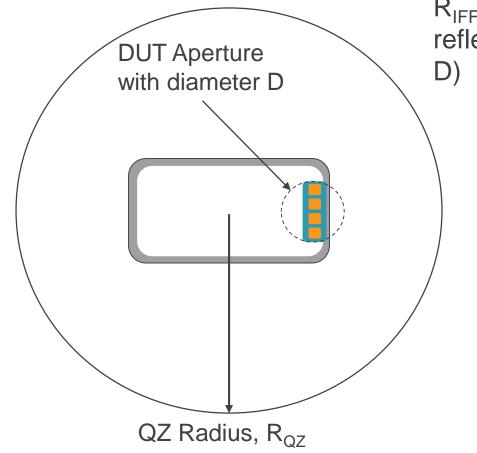
$R_{IFF}$  = focal length (distance between the feed and reflector for a CATR) = 3.5 x size of reflector = 3.5 x (2 x
