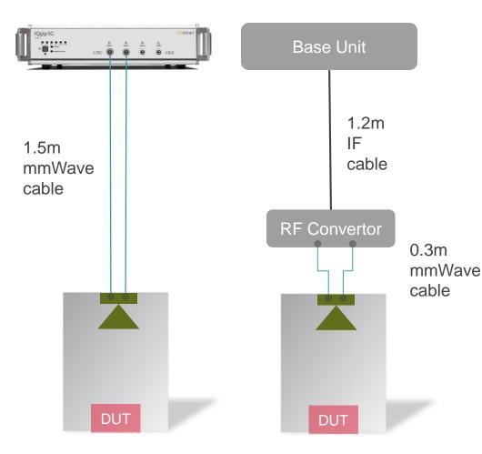
It's true RF converter architecture has less loss due to shorter mmWave cable. However does it matter that much? NO!
