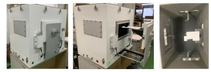
Chamber (DFF) without device positioner (or simple device positioner)
