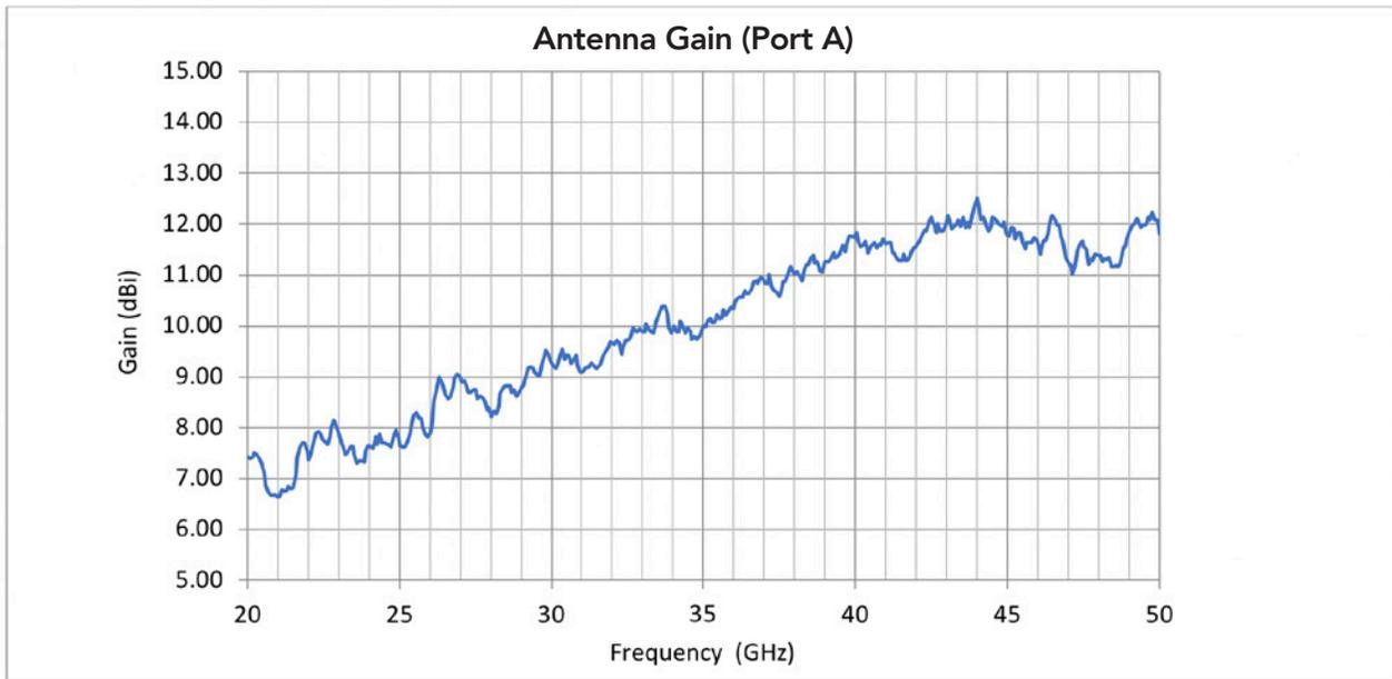
Figure 2: Antenna Gain, Port A
