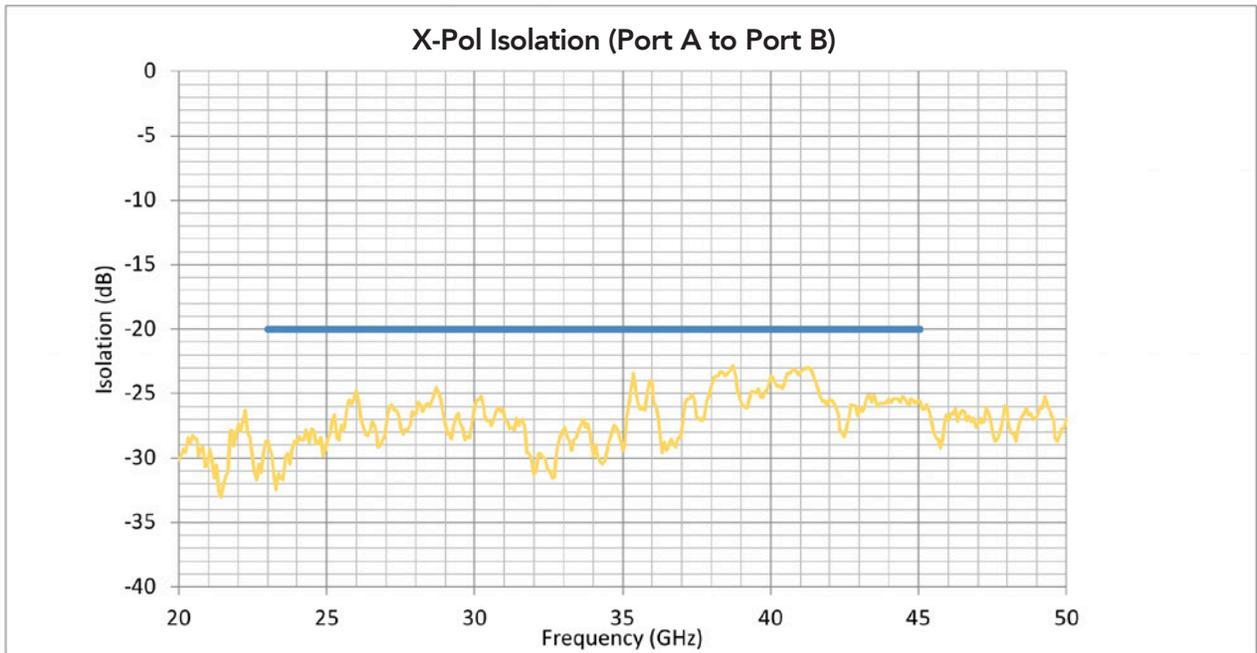
Figure 5: Cross Polarization Isolation Port A to Port B
