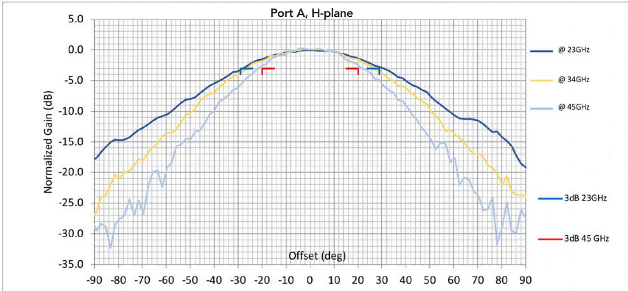
Figure 7: Typical antenna patterns at three different frequencies with Port A, H-plane
