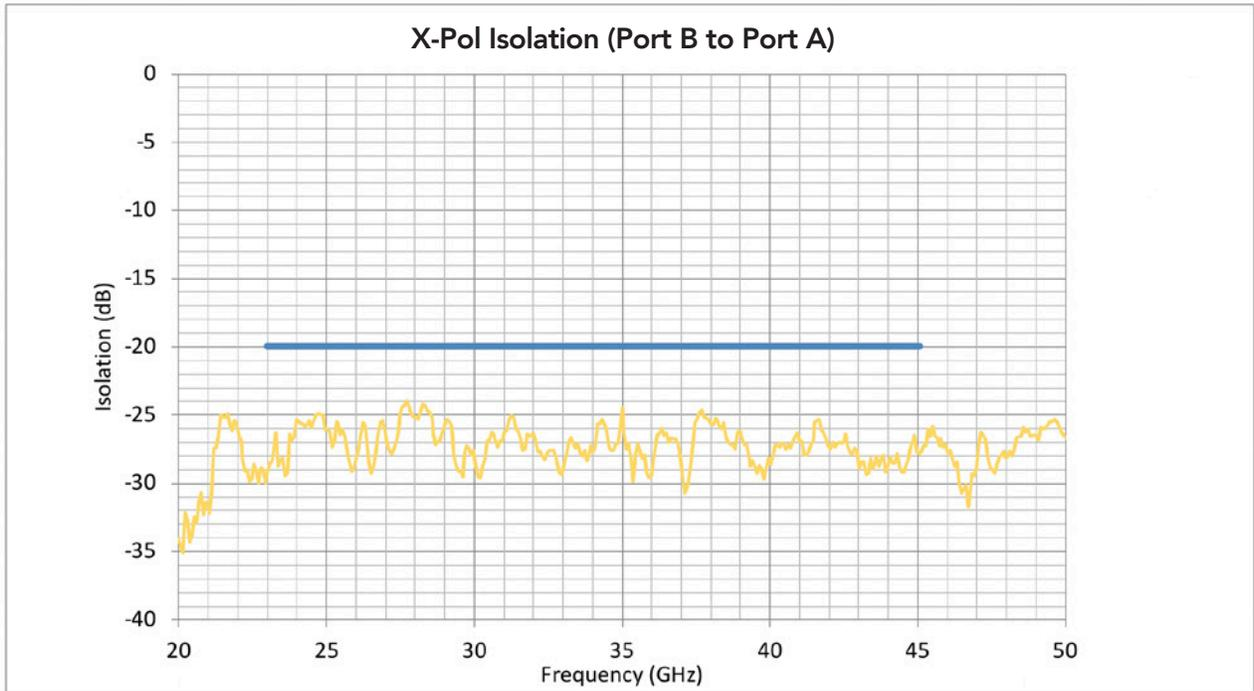
Figure 6: Cross Polarization Isolation Port B to Port A
