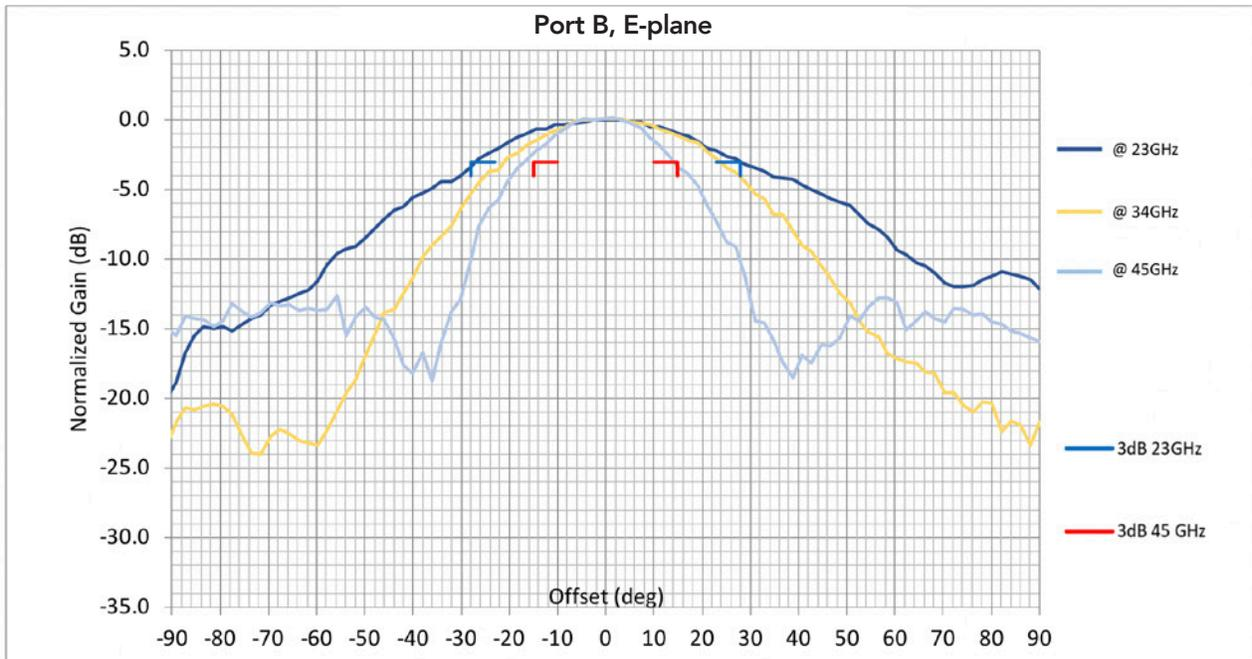
Figure 10: Typical antenna patterns at three different frequencies with Port B, E-plane
