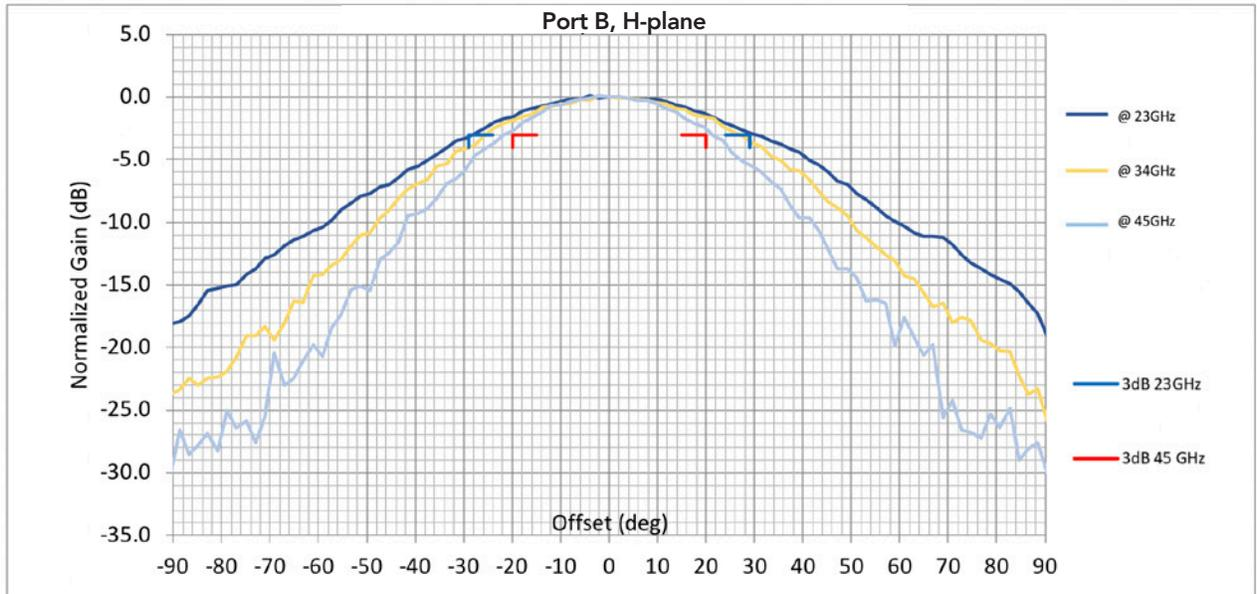
Figure 8: Typical antenna patterns at three different frequencies with Port B, H-plane
