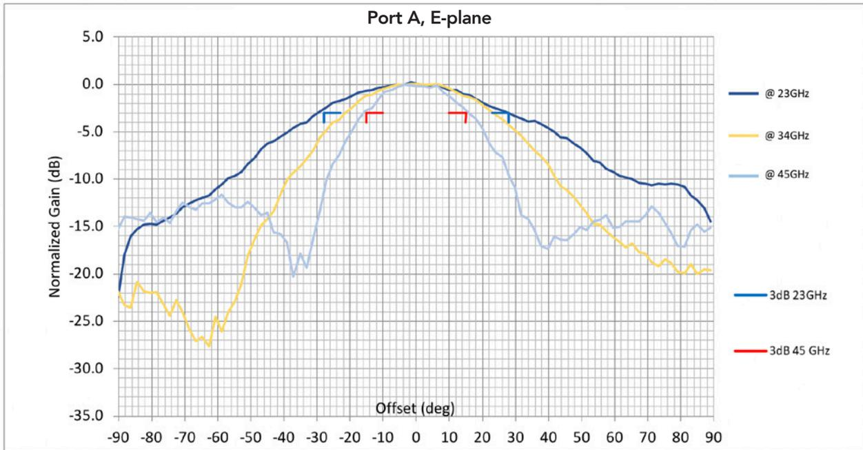
Figure 9: Typical antenna patterns at three different frequencies with Port A, E-plane
