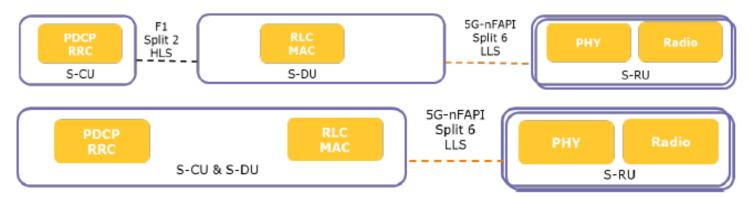
In addition to the SCF FAPI interfaces which provide architecture agnostic APIs between the RF or PHY and higher layer software, the Small Cell Forum is defining the 5G nFAPI message open RAN interface between the S-DU and S-RU(s) over the low layer split 6 fronthaul.
