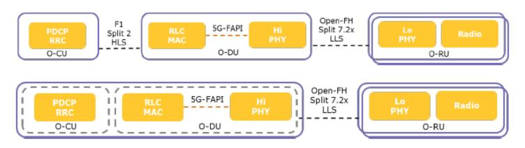
O-RAN has defined a two or three-product solution, with lower layer split option-7.2x and upper layer split option-2. The 7.2x split is defined by the O-RAN open fronthaul Interface between the O-DU and O-RU, which uses the eCPRI protocol specification
