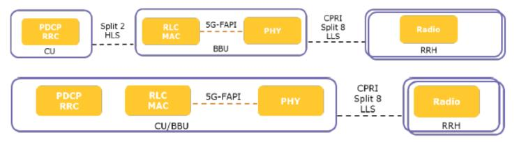
The lowest lower layer split used in the industry is implemented for LTE, and in some early 5G deployments, particularly by MNOs in China where there is ideal fronthaul fiber availability. The fronthaul interface uses a proprietary CPRI specification
