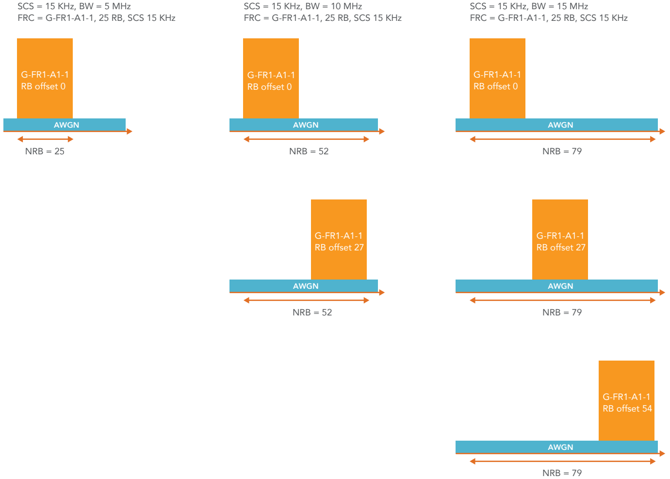
Figure 8. Dynamic range test with FRC waveform RB offset
